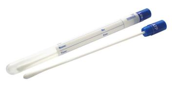
ATP, or adenosine triphosphate is present in all living microorganisms and is used to establish the existence of microbial contamination on food and beverage contact surfaces and microbiological testing in critical areas in clinical, cosmetic and pharmaceutical production facilities to enable earlier quality assurance and release of products.
